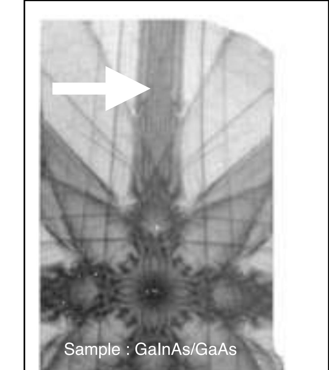
Interpreted as anomalous absorption of Bloch waves in dynamical 2 beams theory
