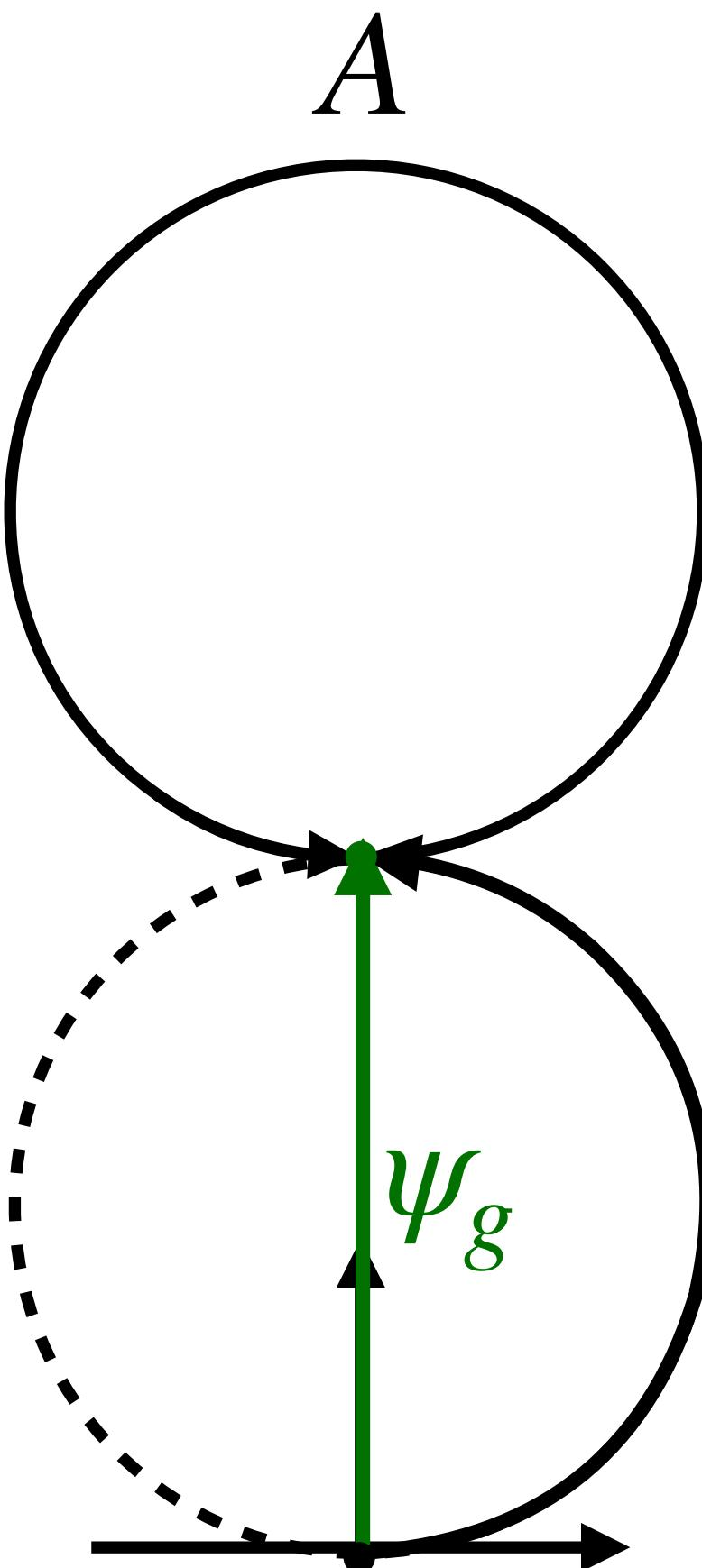
Consider sample thickness  $t = 30\text{nm}$ , with inclined stacking fault with SF vector  $\vec{R} = \frac{1}{4}[110]$
