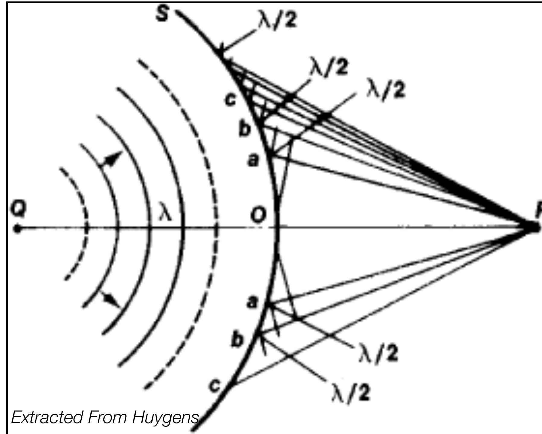
(VI) The integral can be obtained using the first Fresnel zone only :
