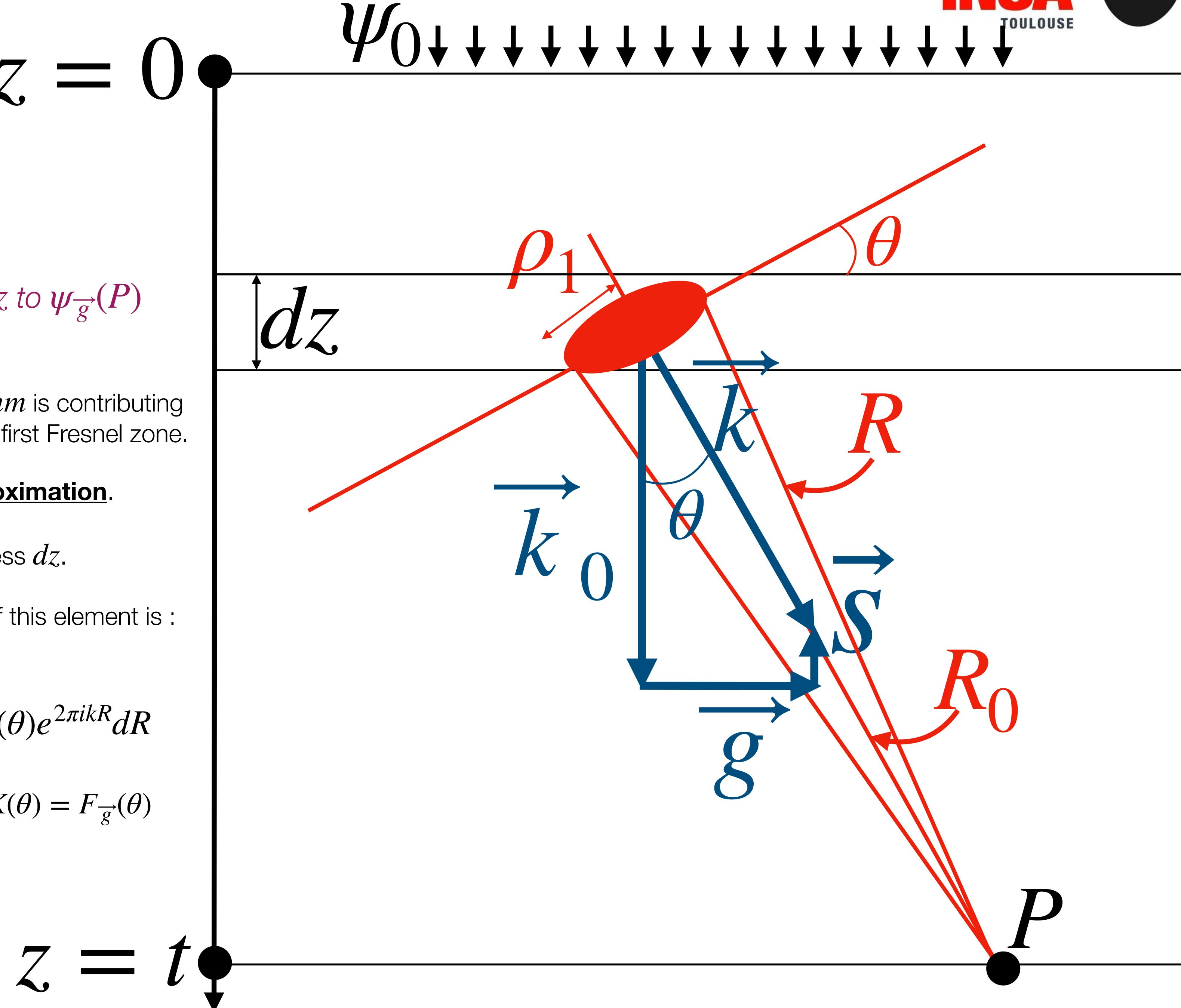
(III) To estimate the diffracted intensity  $I_{\vec{g}}$  we simply have to integrate  $d\psi_{\vec{g}}$  over the thickness
